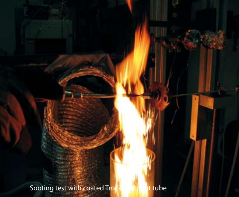
High-temperature non-stick coating on stainless steel pitot tube
