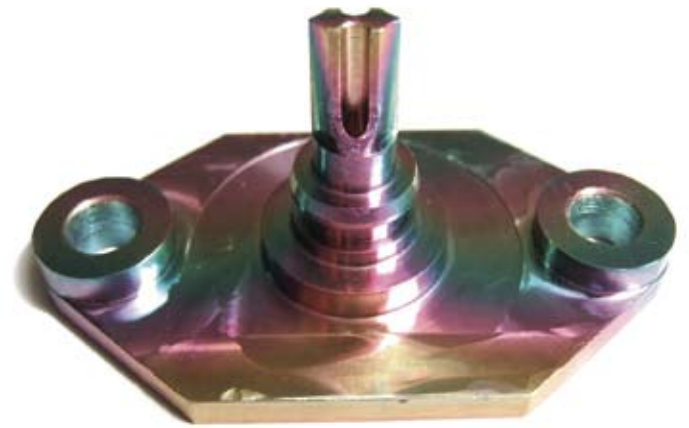
High-temperature non-stick coating on stainless steel pitot tube
