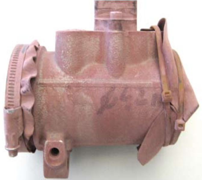
TFI4 flange version venturi after environmental testing
