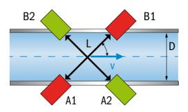
In the time-of-flight technique, sound waves are sent with (A->B) and against (B->A) the direction of flow and accelerated or decelerated in the process. The transit time difference is a measure of the flow velocity.
