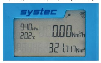
deltawaveSUF is fully parameterised and calibrated at the factory. The 4-button operation is sealed to make deltawaveSUF safe for billing purposes.
