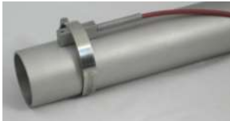
Figure 22: At pipe mounted Pt100
