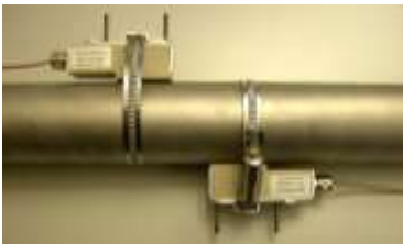
Figure 8: Z-mounting example, only possible without mounting rail (XUC-FW)
