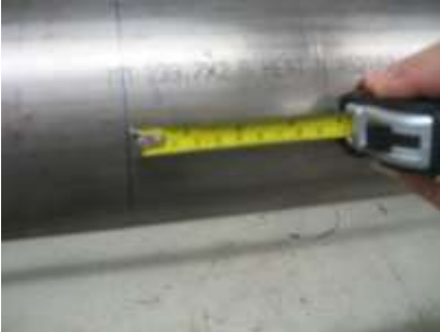
Figure 16: Mark the distance between transducer
