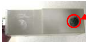
Figure 11: Transducer with an approx. peanut-sized drop of coupling gel
