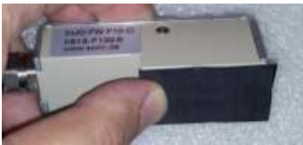
Figure 10: XUC-FW F10 with acoustic coupling pad
