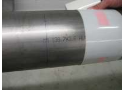
Figure 17: Mark the circumference for the second transducer.
