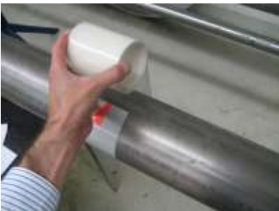
Figure 14: Attaching the template tape
