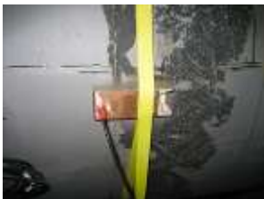
Figure 33: Textile tension bands are recommended for the assembly of the XUC-PW-F05 transducers (temperature limitation)
