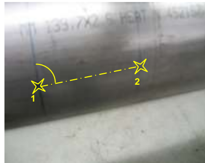
Figure 18: Opposed marks 1 & 2 at the circumference lines
