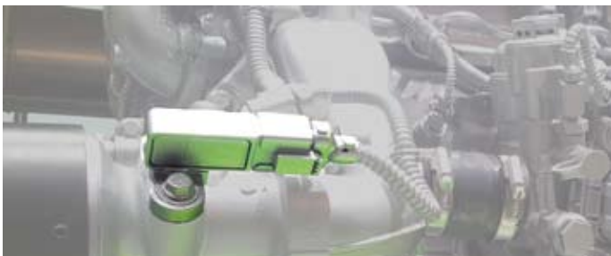
Truckflow pitot tube for air before turbocharger made of plastic with snap-in dp transducer
