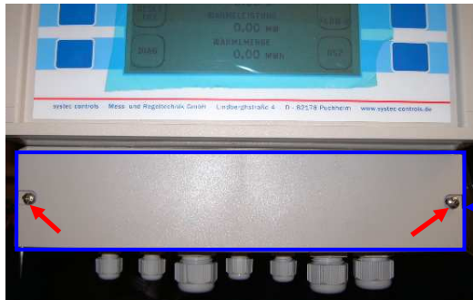
Picture 11 Removing cover plate from cable terminal
