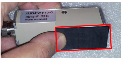
Picture 6 Using acoustic coupling foil
