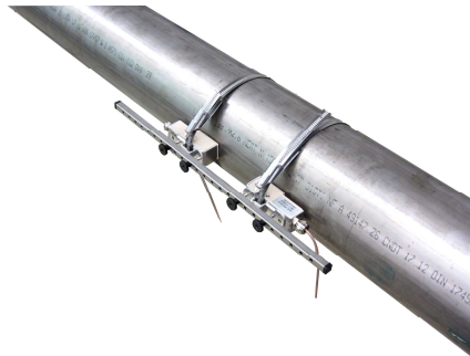
Picture 7 Example Mounted Transducers with spacer bar and mounted at app. 9 o'clock
