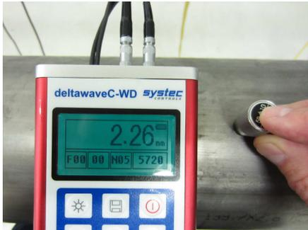
deltawaveC-WD determines the thickness of a structure or a pipe by accurately measuring the time required for an ultrasonic signal to travel through the thickness of the material, reflect from the back or inside surface, and be returned to the transducer. The measured two-way transit time of the ultrasonic together with the specific speed of sound of your material is used to accurately measure the wall thickness. The resolution is 0.1mm
