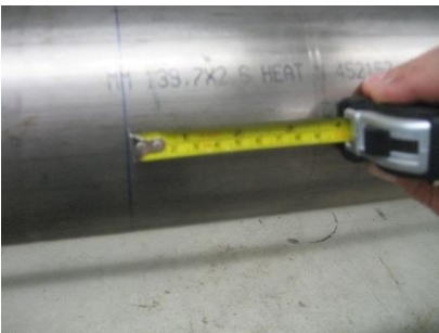
Figure 16: Mark the distance between transducer
