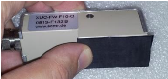
Figure 10: XUC-FW F10 with acoustic coupling pad
