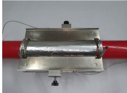
Figure 14: Attaching the damping material between the mounting rails.
