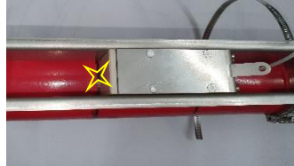
Figure 11: Attaching the transducer to marker 1
