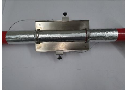
Figure 15: Attachment of the damping material on both sides of the measuring point.
