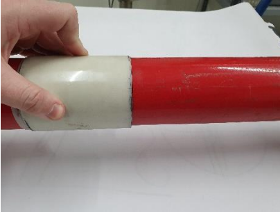
Figure 1: Attaching the plastic stencil 1
