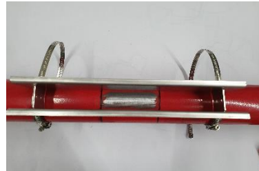
Figure 7: centrally placement of mounting rails
