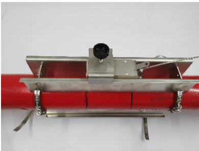
Figure 12: Transducer fixation with mounting bracket
